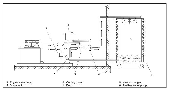
Figure 4-12 Cooling Tower System
